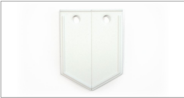
Figure 14: Raw, unfinished EOS PA 2200 sample
