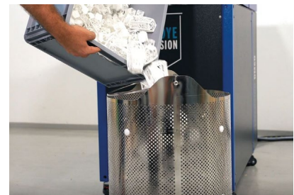
Figure 6-8 LTR: The DeepDye Coloring (DDC) process: scanning a color cartridge, inserting the cartridge into the basket, filling the basket with parts
