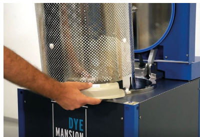
Figure 6-8 LTR: The DeepDye Coloring (DDC) process: scanning a color cartridge, inserting the cartridge into the basket, filling the basket with parts
