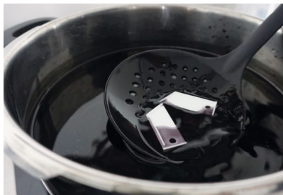
Figure 2-4: Pouring textile dye into the water, putting the parts in the pot, drying the parts
